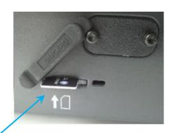
d. Tilt down the SIM card cover to its original position.
