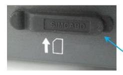
Position the SIM card with its goldcontacts facing down. (There is a symbol of SIM Card with its arrow on the front panel to ensure the correct orientation of the SIM Card when it is being inserted.)
