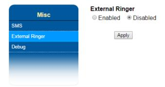
Click **Enabled** to activate the external ringer (or buzzer) when there is an incoming call. The external ringer's wires are connected to Pin 9 and Pin 10 of the BDU GPIO Output Port.
