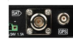
1. Plug the two RF cables to the RF cable connectors on the Base Terminal
